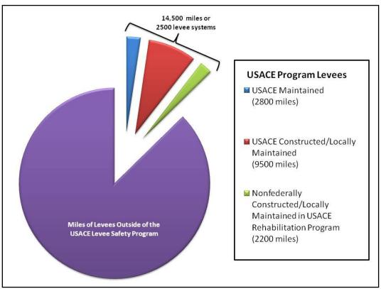
Figure 9-4. U.S. Levee System
